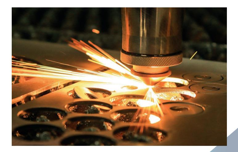
Laser cutting is the fastest and most efficient way of cutting metals.
